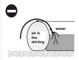
Fill the pool with water using air-filled skirting (exclusion of guarantee).
