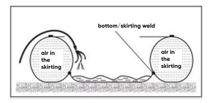
2. Stop filling when the water reaches the top of the bottom/skirting seam. The shape of the pool is not yet final.
