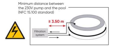
You must use a socket fitted with a 30mA differential circuit breaker. <u>More details on pages 18 and 19 of this leaflet.</u>
