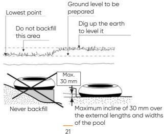
It is particularly important for the ground to be stable, compact and free of anything that could damage the pool. To correct any unevenness in the floor, spread, level and compact a layer of washed 0.2 mm crushed sand approximately 2 cm thick before installing the floor mat.
